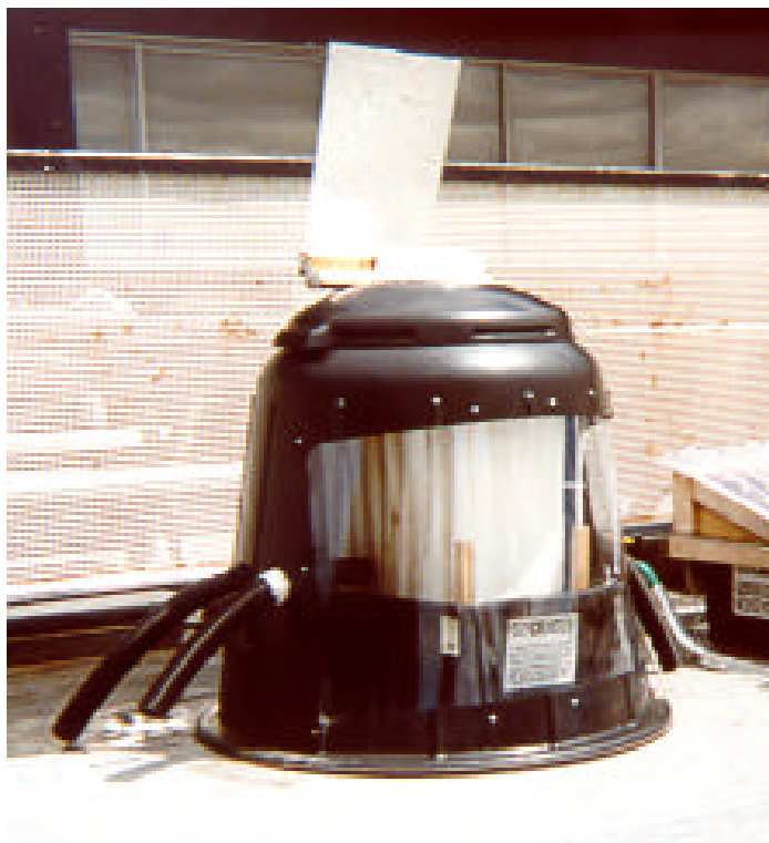
Plate 2. Prototype evaporator showing north facing transparent window, with wick system behind, and reflector on top which increases sunlight onto solar powered fan.
