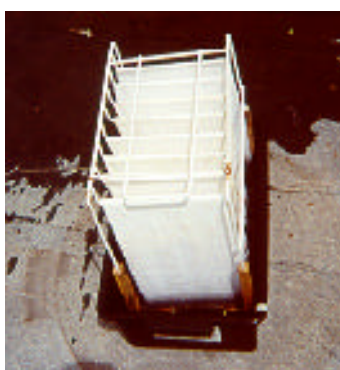
Plate 1. View from above the wick system used in the prototype evaporator.
