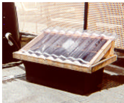
Plate 3. Evaporator used as a control during testing of the prototype.
